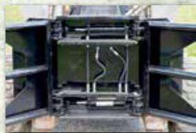
Features dual cylinder system and rigid frame for better gripping power.
